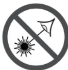
**DO NOT direct the laser beam at persons or animals and do not stare into the laser beam yourself. This laser measure produces class 2 laser radiation and complies with 21 CFR 1040.10 and 1040.11 except for deviations listed in the following table.**
