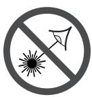
**Do not direct the laser beam at persons or animals and do not stare into the laser beam yourself.** This tool produces laser class 2 laser radiation and complies with 21 CFR 1040.10 and 1040.11 except for conformance with IEC 60825-1 Ed. 3., as described in Laser Notice No. 56, dated May 8, 2019.
