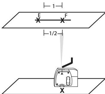
10. Mark the up beam on the ceiling, Mark F. You should have two marks on the ceiling.
