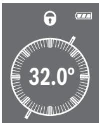
Inclination measurement is used to measure a slope or incline. The left side of the laser measure serves as the reference level for inclination measurement.
