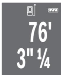
Watch the numbers move in real time as you move the laser measure towards or away from the object you are aiming at.
