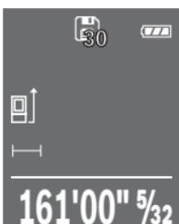
If there is no value yet saved to memory, "0'00" is shown at the bottom of the display and "0" at the top.
