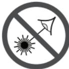
**DO NOT direct the laser beam at persons or animals and do not stare into the laser beam yourself.** This laser measure produces class 2 laser radiation and complies with 21 CFR 1040.10 and 1040.11 except for deviations pursuant to Laser Notice No. 50, dated June 24, 2007. This can lead to persons being blinded.
