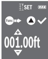
Set the desired length by pressing the function button **7** [**Func**] to scroll through the digits you want to change and by pressing the plus button **3** [ $\blacktriangleright$ ] or minus button **8** [ $\blacktriangleleft$ ] to change the value of each digit.
