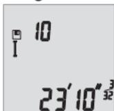
The number of the measured value is displayed after and the respective measured value is displayed underneath.
