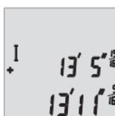
Press button **6** to add measured values or press button **3** to subtract measured values. “+” or “-” will appear in the middle of the display. Take another measurement. The current measured value will be shown at the bottom of the display, and the previous measured value will be shown above it.
