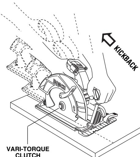
**Never place your hand behind the saw blade.** Kickback could cause the saw to jump backwards over your hand.
