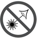
**Do not direct the laser beam at persons or animals and do not stare into the laser beam yourself.** This tool produces laser class 2 laser radiation and complies with 21 CFR 1040.10 and 1040.11 except for deviations pursuant to Laser Notice No. 50, dated June 24, 2007. This can lead to persons being blinded.
