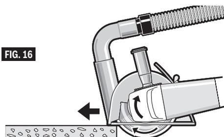
When cutting especially hard material, e. g., concrete with high pebble content, the dry diamond wheel can overheat and become damaged. This is clearly indicated by circular sparking of the rotating dry diamond wheel. In this case, interrupt the cutting process and allow the dry diamond wheel to cool by running the tool for a short period of time at the maximum speed with no-load.
